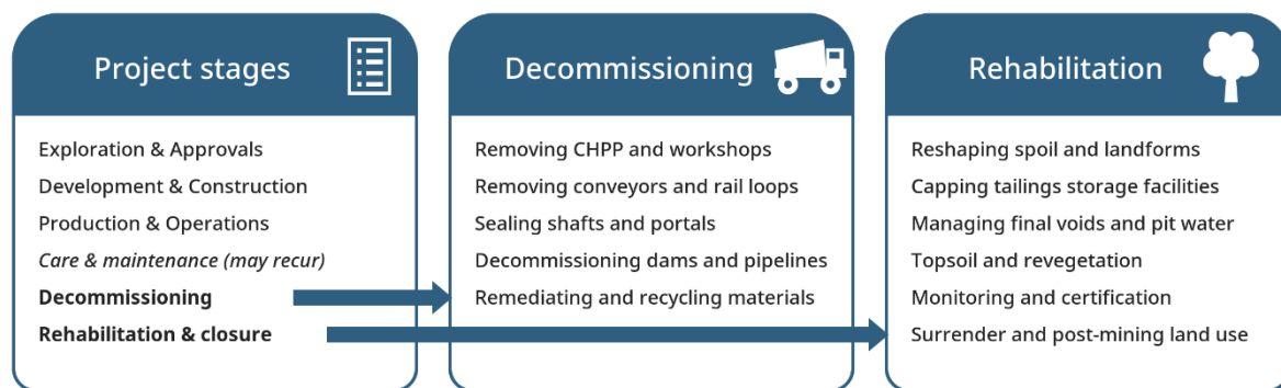
Figure 1: Stylised end stages of a coalmining project
