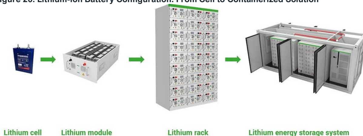
Figure 26: Lithium-ion Battery Configuration: From Cell to Containerized Solution
