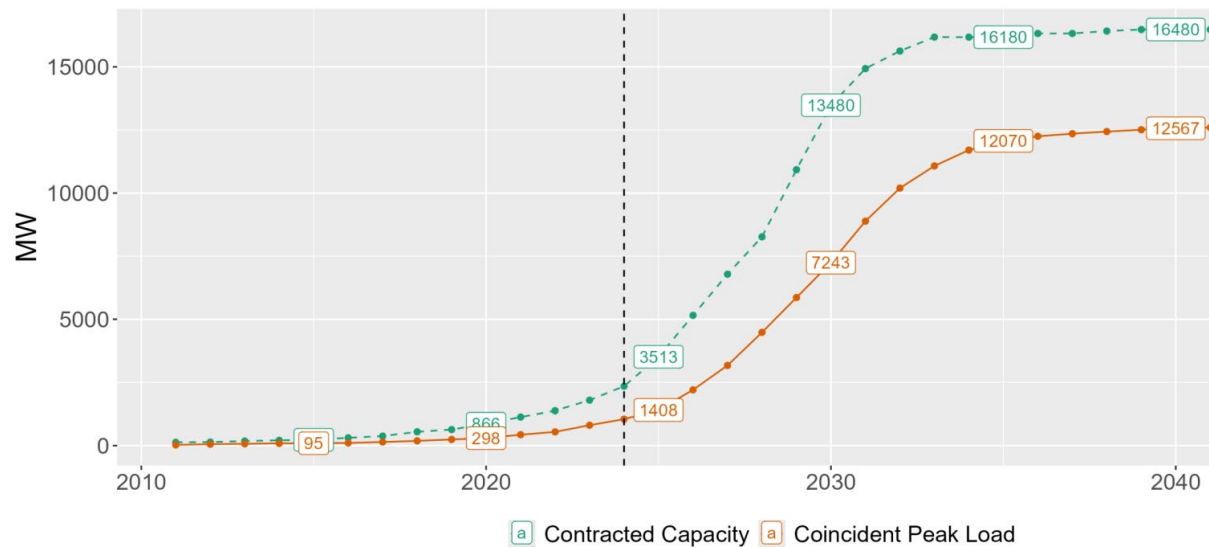
Figure 5: Northern Virginia Electric Cooperative (NOVEC)’s Data Center Load Forecast, As Submitted to PJM Interconnection
