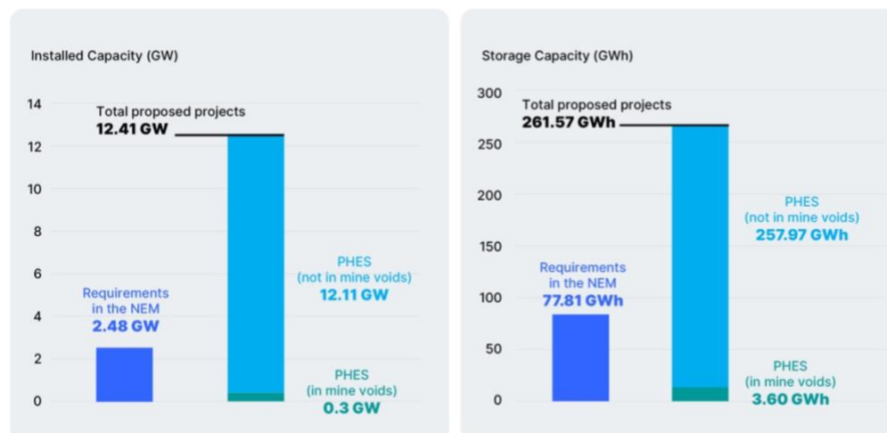
Figure 13: Deep storage duration projects proposed in the NEM by 2050, versus AEMO requirements under Step Change scenario
