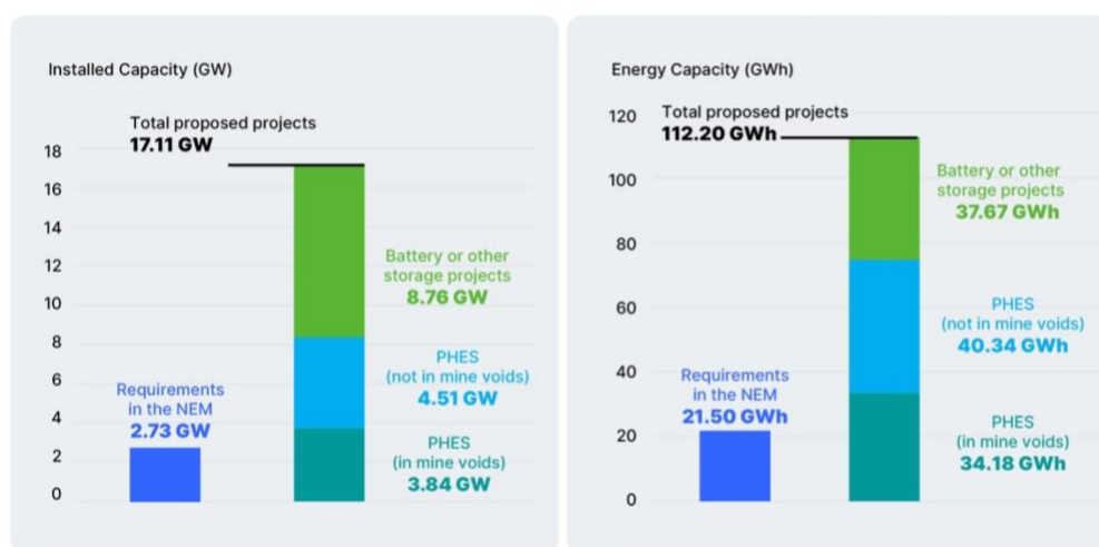
Figure 12: Medium storage duration projects proposed in the NEM by 2050, versus AEMO requirements under Step Change scenario
