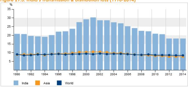
Figure 29.3: India's Transmission & Distribution loss (1990-2014)
