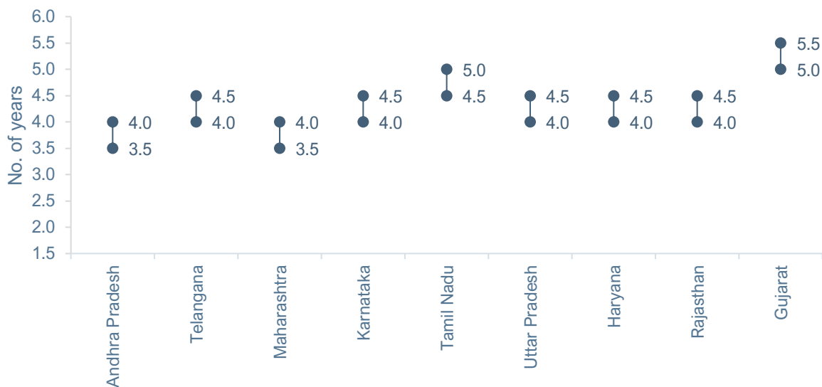
Figure 5: Payback Period of Industrial Solar Installations in the CAPEX Model in India (March 2023)
