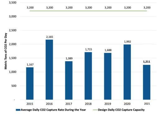
Figure 16: Projected vs Actual Boundary Dam CO<sub>2</sub> Daily Capture Rate
