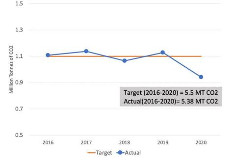
Figure 18: Target vs Actual Capture Rate of Quest CCS Plant (2016–2020)
