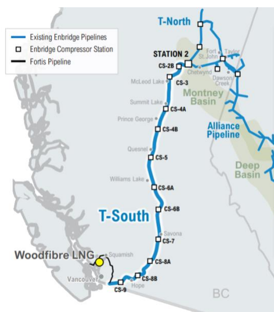
Figure 5: Pipeline System Intended to Source Natural Gas from the B.C. Montney for the Proposed Woodfibre LNG Facility
