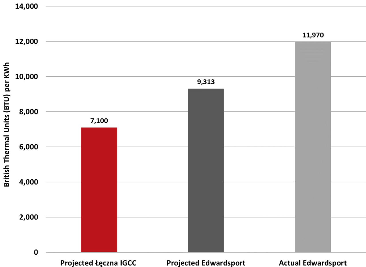
A higher heat rate will mean Łęczna will be more expensive to operate as it will need to burn much more coal to produce the same amount of electricity.
