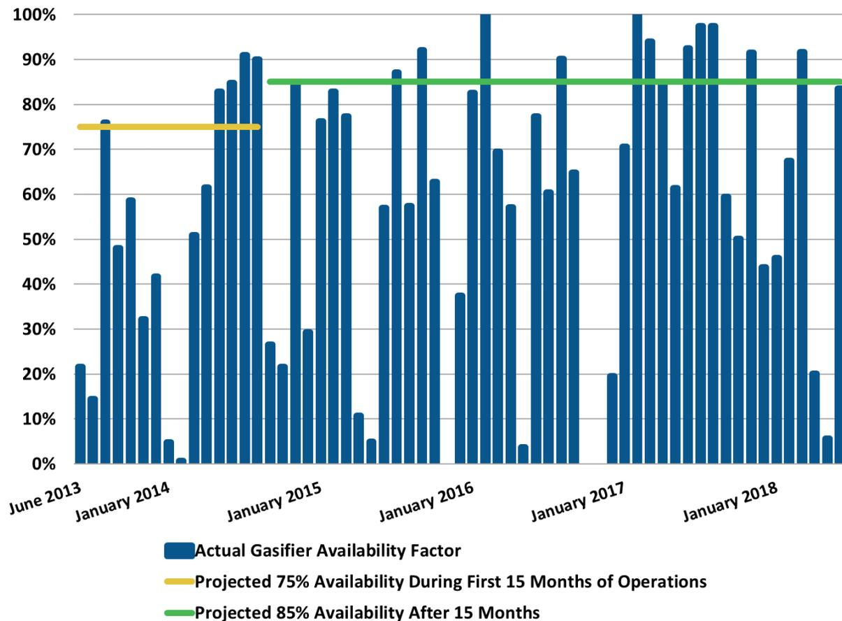
Another commonly used measure for evaluating a power plant's operating performance is its Equivalent Forced Outage Rate (EFOR). EFOR is a measure of the probability that a unit will not be available, accounting for both (1) forced outages when the entire plant is out of service and (2) derating of the plant below its rated full power net capacity (that is, where the plant is available to generate but only at a lower output due to unplanned equipment problems or technical issues).
