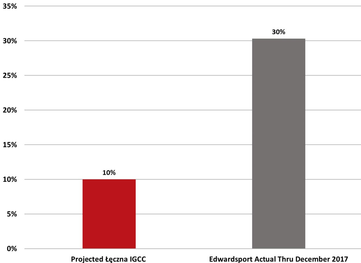
Higher parasitic loads can hurt plant performance (and customers) in several ways. First, the plant will either have to be built larger to produce the same 488 net MWe of output, or its actual net MWe will be substantially lower than proposed. Building a bigger power plant will increase the cost of building the plant. At the same time, the plant will have to burn substantially more fuel in order to both operate the gasification system equipment and sell its net output into the grid.
