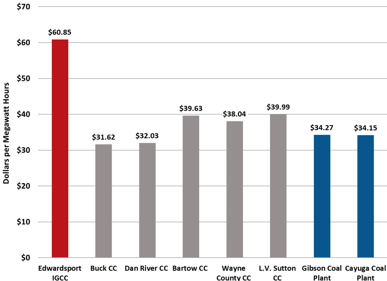
Edwardsport's fuel costs are relatively low compared to the other plants in Figure 7. However, its non-fuel O&M expenses are much higher. It appears that these extremely high non-fuel O&M expenses are due, in large part, to the high cost of operating and maintaining the plant's gasification systems.
