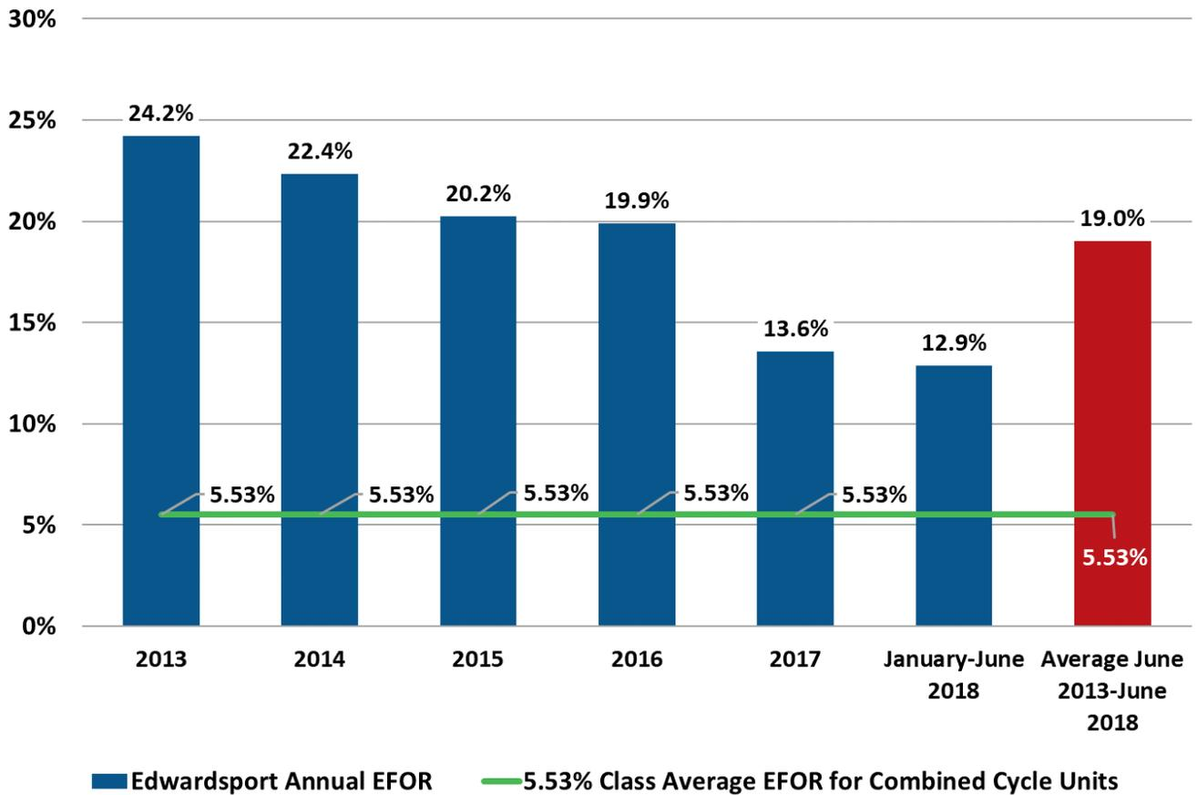
Edwardsport's average 19.0% EFOR from June 2013 through June 2018 was more than three times the average EFOR of the industry comparison group.
