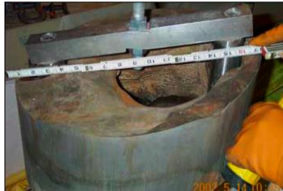
The hole in the Davis-Besse reactor head, 2002
